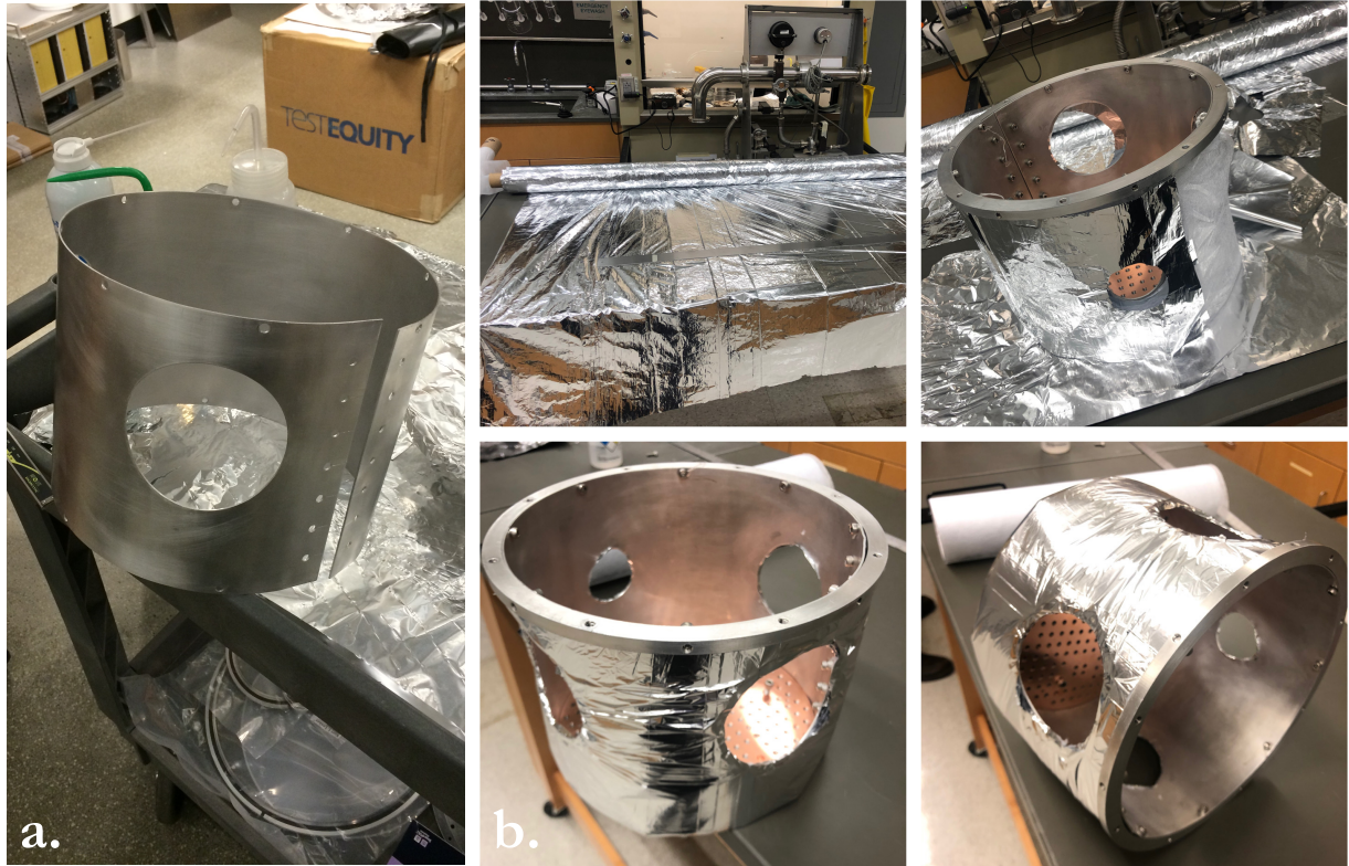
Figure 5.6: 35K shield: a. First, we drill hole patterns in the aluminum sheet and roll it into a cylinder, b. we cover the surface of the shield with several repeated layers of Mylar and insulator
